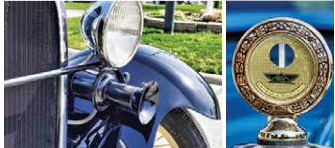
"Ah-oo-gah" horn; Radiator cap with temperature gauge
