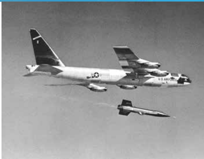
X-15 Air-drop from Boeing NB 52A Stratofortress B52-003 Glide Flight
